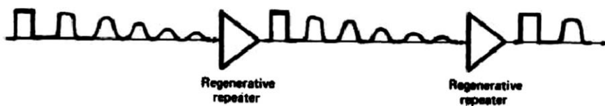
Figure 1.5 signal regeneration in a digital repeater line
